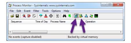
If you are looking for an issue related to registry accesses, then enable ONLY the *Show Registry Activity* button. If you are looking for file access issues, use the second *Show File System Activity* button. The other three buttons are for Network Activity, Process and Thread Activity, and Profiling Events, respectively. Again, simplicity will save you time here, so you should always disable any events that you don't care about first.
